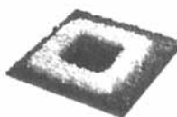
FIGURE 5 The piezoresponse image of a large-scale poled area (scan area: 6\mu\text{m} \times 6\mu\text{m} ). See color plate XII at the back of this issue.
